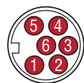
Integral D6 connector (male) as viewed from the end of the sensor
