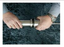
**3.4** Assemble the top and bottom turning clockwise.
