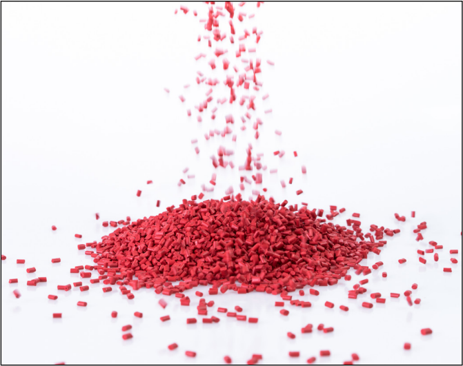
Fig. 2: Plastic granulate for injection molding or extrusion
