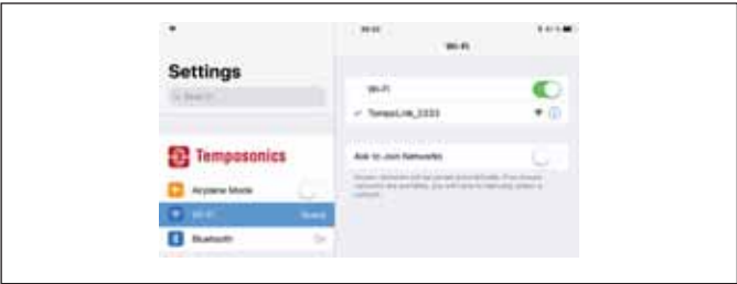
Fig. 83: Choose the network “TempoLink_xxxx” in the Wi-Fi settings of the Wi-Fi-enabled device
