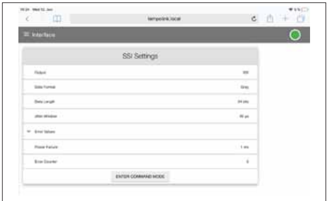
Fig. 92: Configuration of SSI settings
